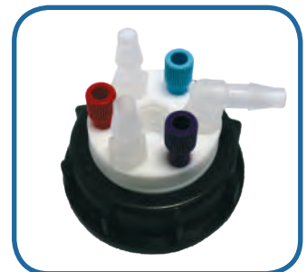
SW55-3-C-3L : 3 entries 1/8", a charcoal cartridge emplacement and 3 tube fittings
