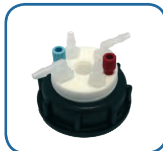
SW60-2-C-4L : 2 entries 1/8", a charcoal cartridge emplacement and 4 tube fittings
