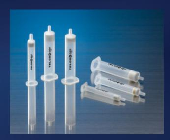
Reversed phase (non-polar) SPE remains a popular SPE approach due to its applicability to a wide range of compounds. Provided the analytes have sufficient non-polar (hydrophobic) character, extraction of single compounds or multiple analyte suites is achieved.
