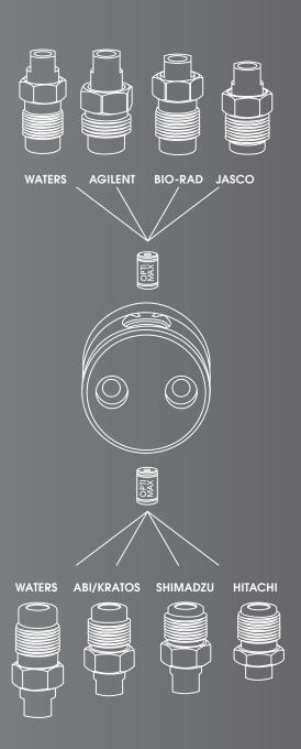
A single Opti-Max cartridge is interchangeable across multiple pump brands and can function in either the inlet or outlet position.
